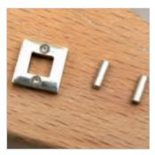
The two pieces of wire should fit both the top section of the ring and into the upper side of the shank.
