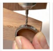
Measure the top of the ring shank against the top piece drilled in step 5. Mark the position of the two holes and then drill matching indentations.
