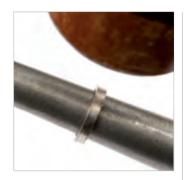
Form the annealed palladium wire for the ring shank around a ring mandrel. Make the ends meet very tightly and neatly with a rawhide mallet and flat-nosed pliers if necessary. Palladium solder is not as smooth flowing as gold or silver, so be sure the seam is as tight fitting as possible.
