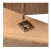
5 Measure and mark the centre point along two sides of the base of the central piece. Drill indentations into these marks but do not drill all the way through: approximately 1mm (½2in) depth is required. If necessary, extend the width of the holes with the 0.7mm (½2in) burr until the two wire pieces slot in tightly and securely.
